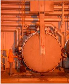
**Figure 4.4: Autoclaves where AAC is pressurized and cured**
